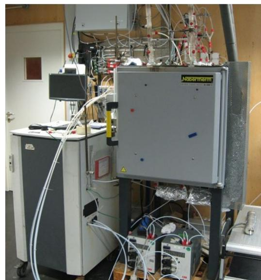
Laboratory micro reactor operated at USTUTT (right) with continuous mercury analyzer installed in an air conditioned cabinet (left)
